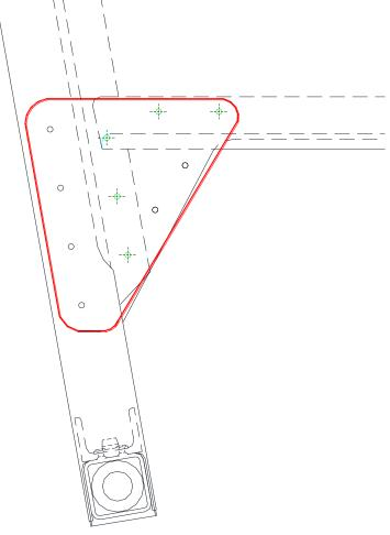
Figure 3 – Seat back patch location, LHS of seat shown. View is from behind seat.
