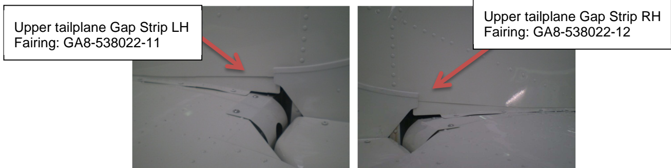
Figure 1: Horizontal Stabiliser connects to Fin Assembly
