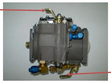
Figure 1: Throttle and Mixture control lever locations
