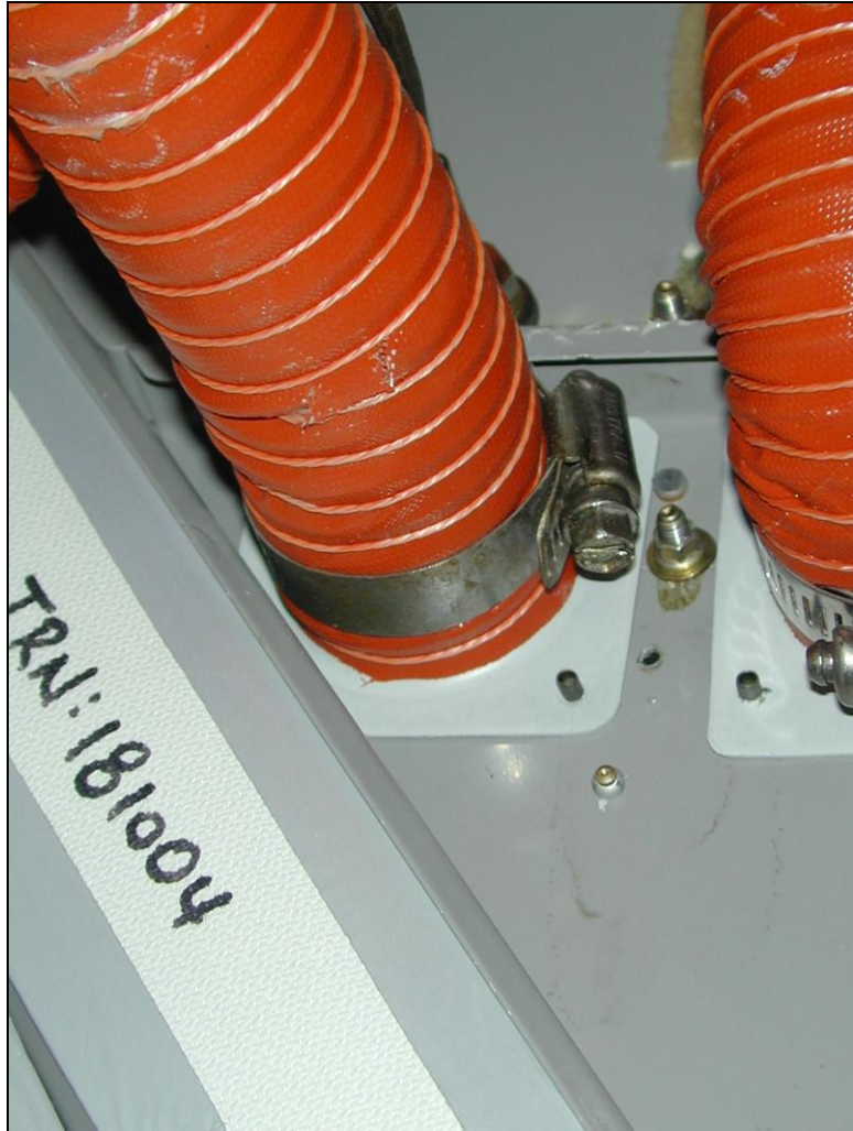
Figure 5: Completed RHS modification viewed from inside the aircraft.
