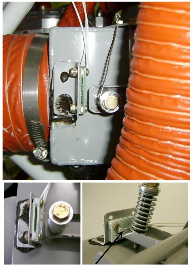
Ensure sensor element is placed in front of metal portion of the door return spring bracket Figure 6: Switch bracket installation.
