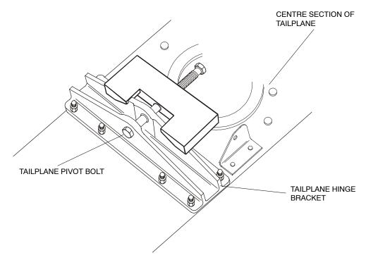
Figure 2 Tailplane Pivot Bolt Extractor Tool Installation
