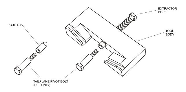
Figure 1 Tailplane Pivot Bolt Extractor Tool Kit
