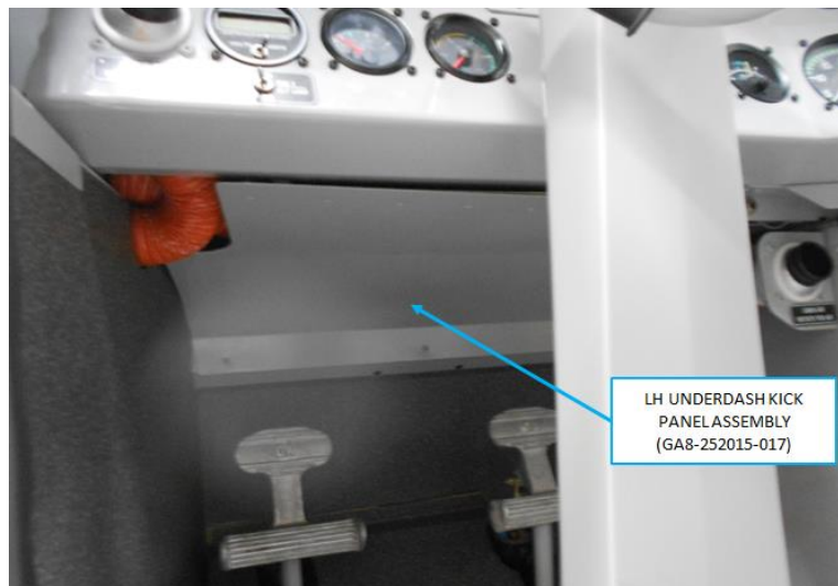
Figure 1: LH Underdash Kick Panel Location
