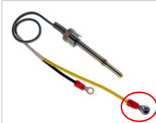
Figure 3 – Pictorial view of CHT Bayonet Probe. Note screw fitted to yellow lead ring terminal (circled).
