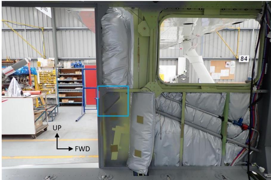
**Figure 17:** Removal of interior trim and insulation. View looking at the interior structure of the aircraft's port side fuselage wall.
