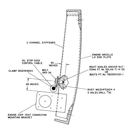
Installation of Oil Stop Cock Control Cable Clamp - Scrap View Figure 2
