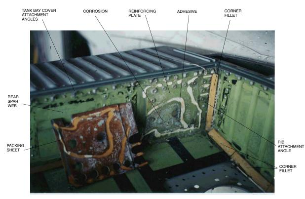
Figure 2 – Inboard Tank Bay – RH Wing
