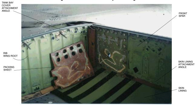
Figure 5 – Inboard Tank Bay – RH Wing
