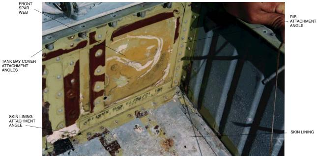
Figure 3 – Outboard Tank Bay – LH Wing
