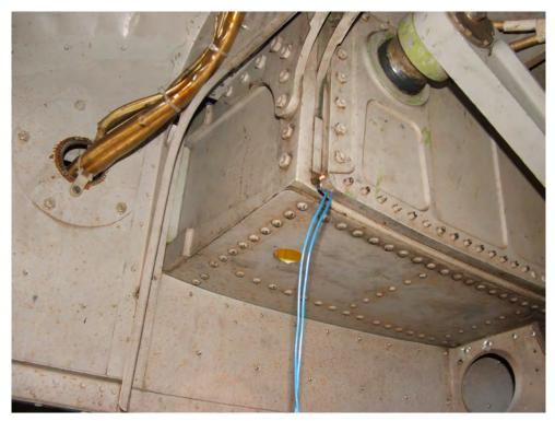
LIGHT SOURCE INSERTED INTO STUB WING BAY
