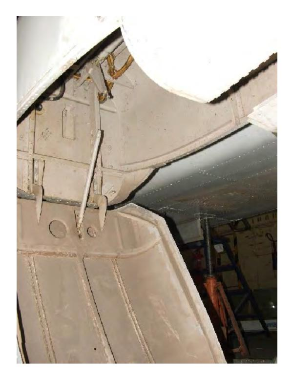
Figure 1 LH Landing Gear Pod Door - Disconnected (RH Similar)
