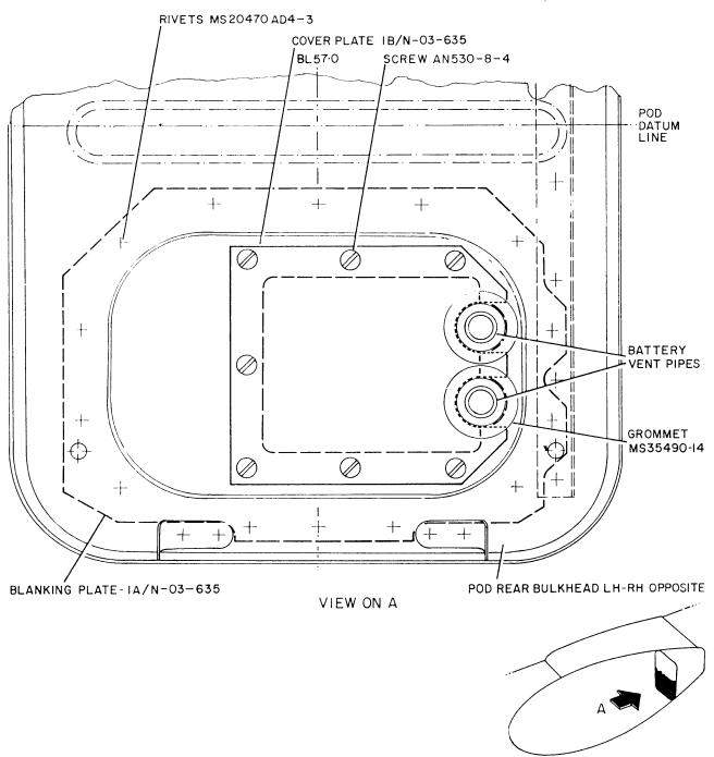
Blanking and Cover Plate LH Side Installation Figure 2
