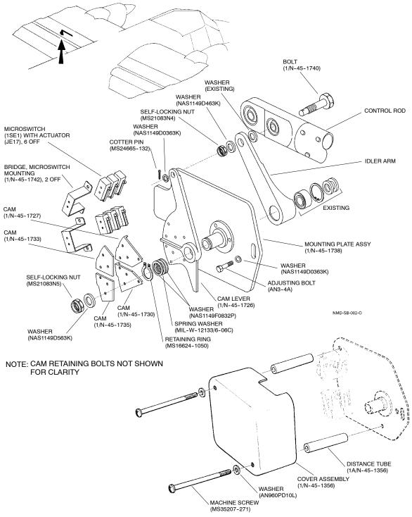
Figure 5 Cam/Microswitch Assembly (Mod N874)
