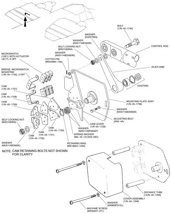
Figure 2 Cam/Microswitch Assembly (Mod N835)
