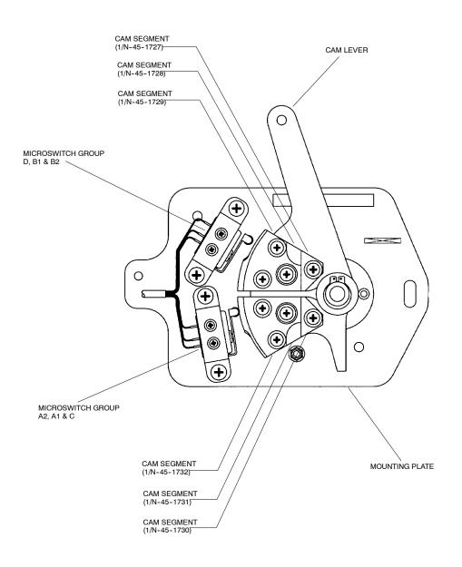
Figure 3 Cam/Microswitch Assembly (Mod N835)
