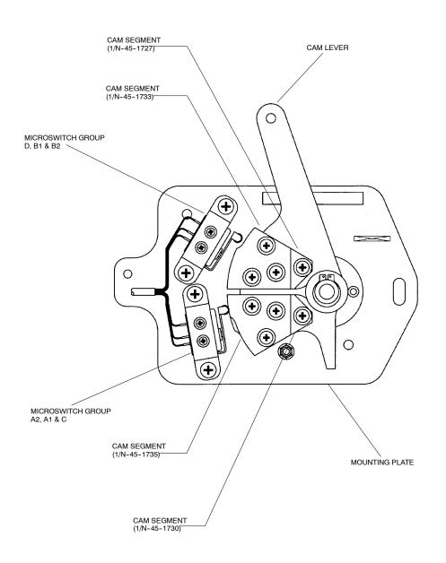
Figure 6 Cam/Microswitch Assembly (Mod N874)
