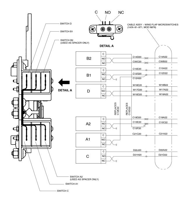
Figure 7 Mod N874 (N24) Microswitch Positions and Schematic Wiring Diagram
