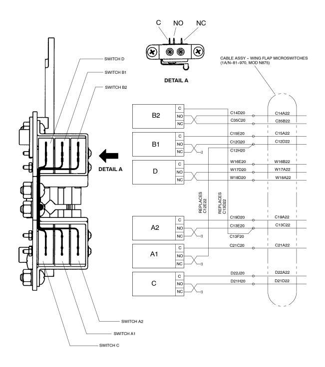
Figure 4 Mod N835 (N22) Microswitch Positions and Schematic Wiring Diagram
