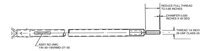
Figure 1 Rework of Horizontal Stabiliser Trim Tab Control Rods
