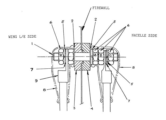
Figure 1 Starter Cables and Stud Assembly
