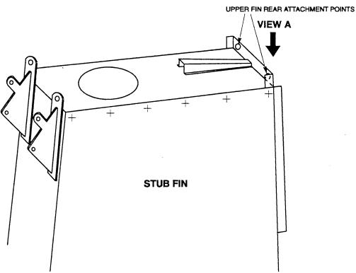
Figure 1 - Upper Fin to Stub Fin Attachment
