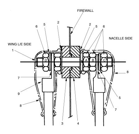
Figure 1 Generator Cables and Stud Assembly
