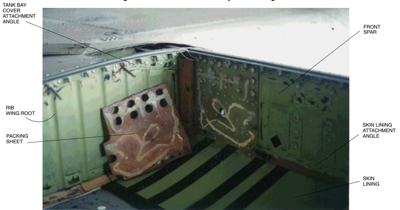
Figure 5 – Inboard Tank Bay – RH Wing
