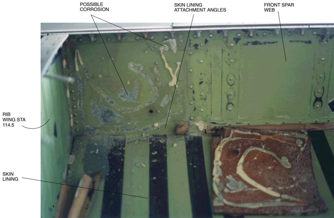
Figure 4 – Outboard Tank Bay – RH Wing
