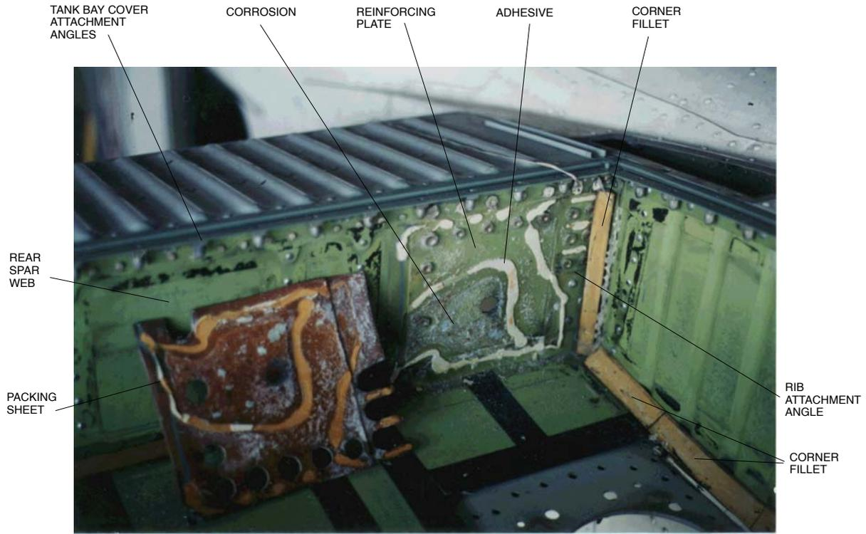
Figure 2 – Inboard Tank Bay – RH Wing
