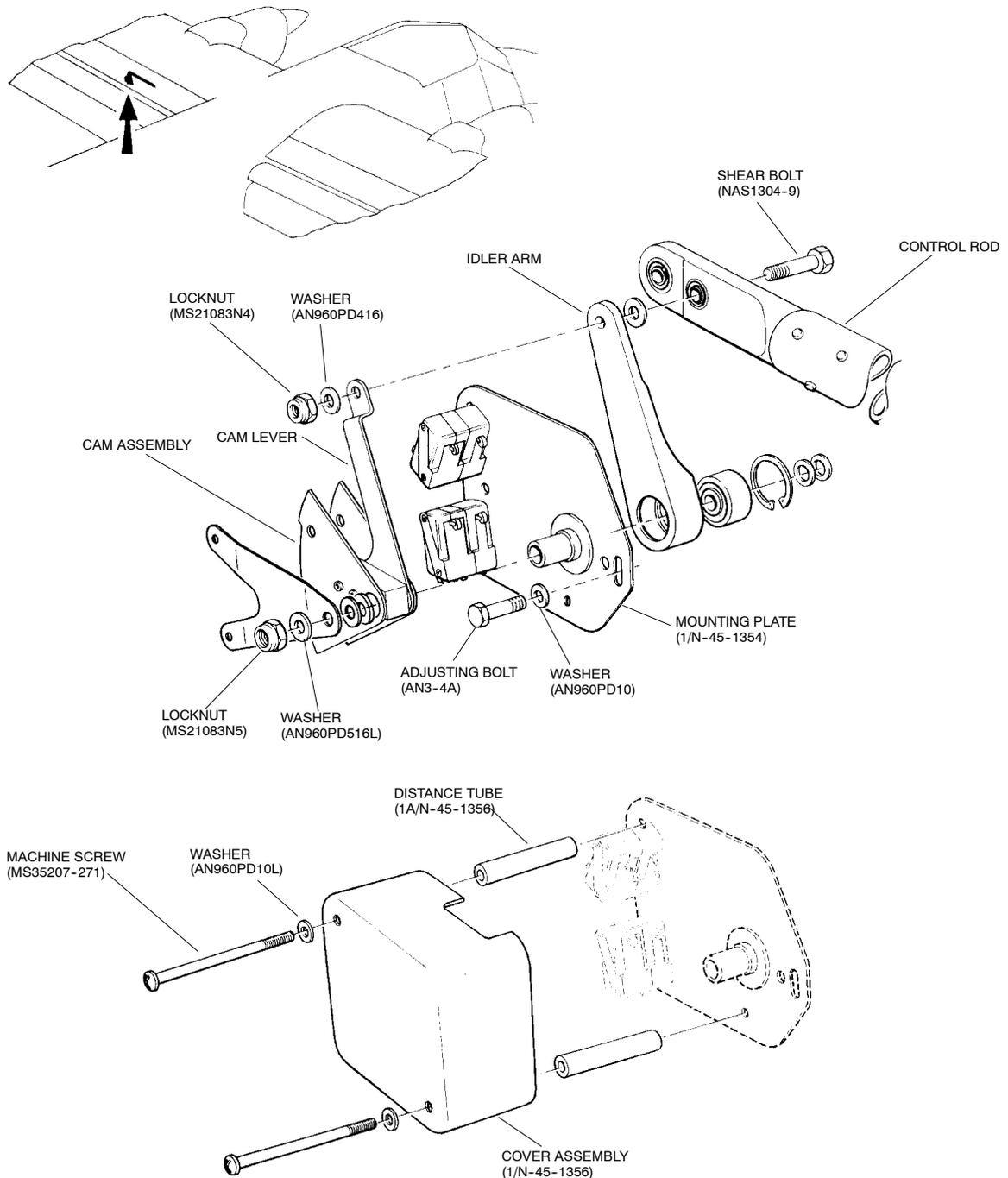
**Figure 1 Existing Cam/Microswitch Assembly (Post-Mod N46 or N124)**
