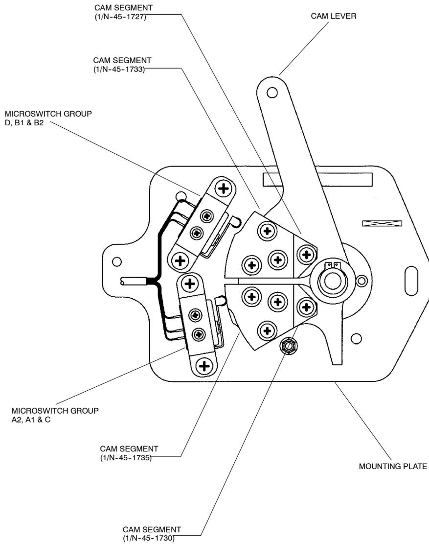
**Figure 6 Cam/Microswitch Assembly (Mod N874)**
